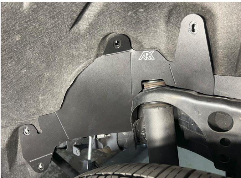
Picture of secured Rear Splash Guards to the frame
